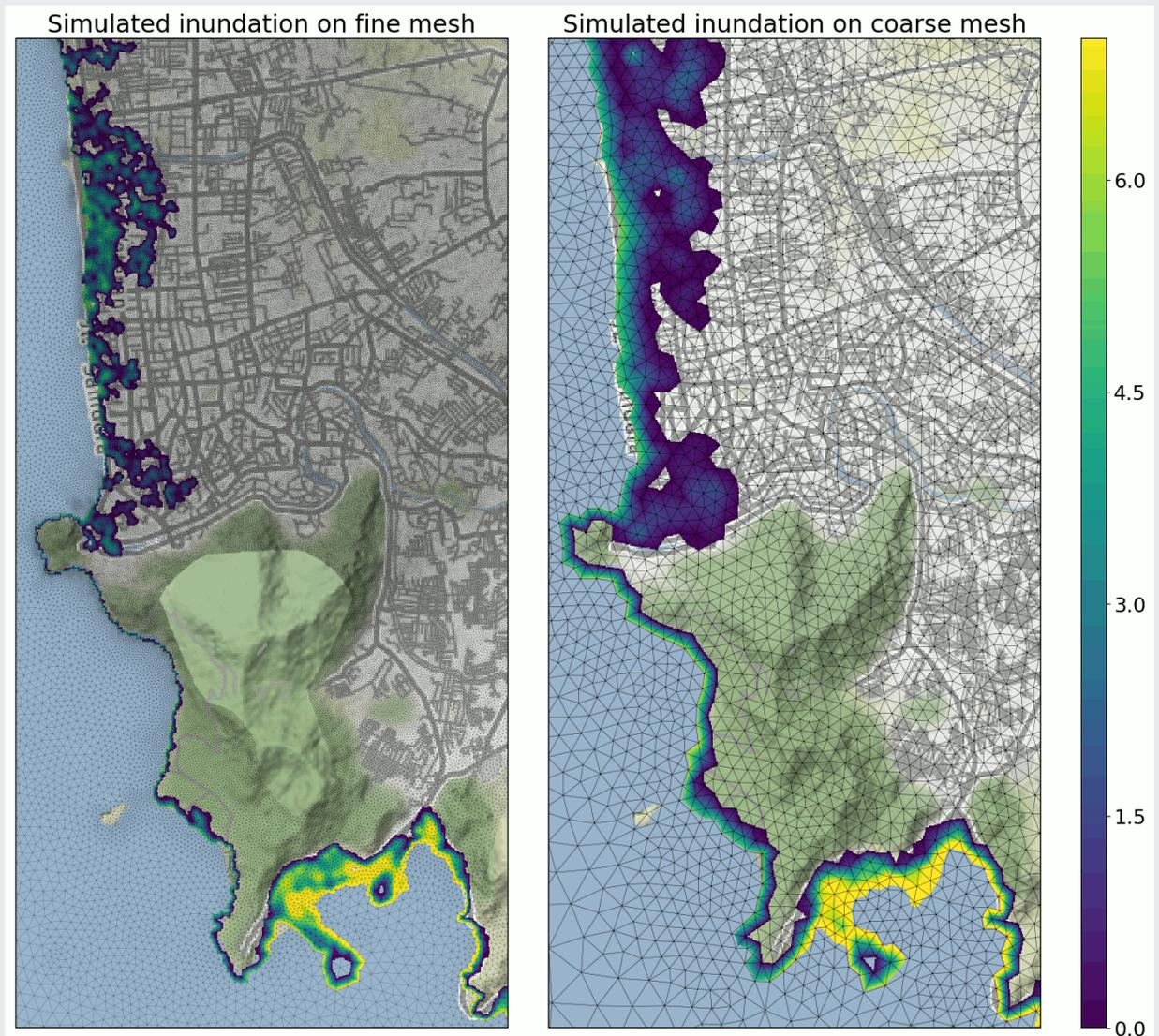
*Inundation maps for both a precise and a coarse mesh. The faster coarser calculation already provides valuable information.*
