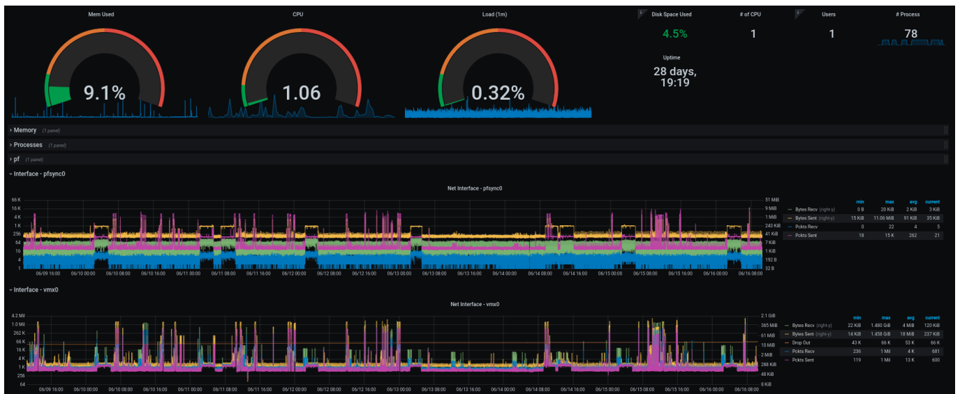
Figure 15: pfSense system dashboard at LRZ
