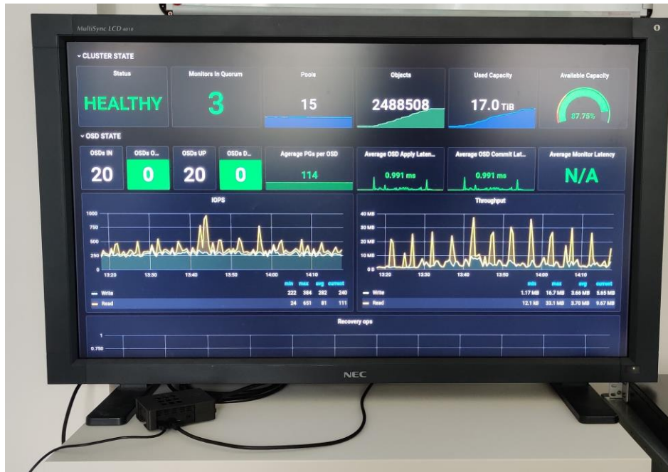
Figure 6: CEPH Dashboard displayed on large screen with Raspberry Pi
