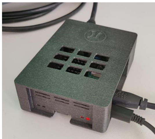
Figure 7: Raspberry Pi computer with custom image for monitoring display
