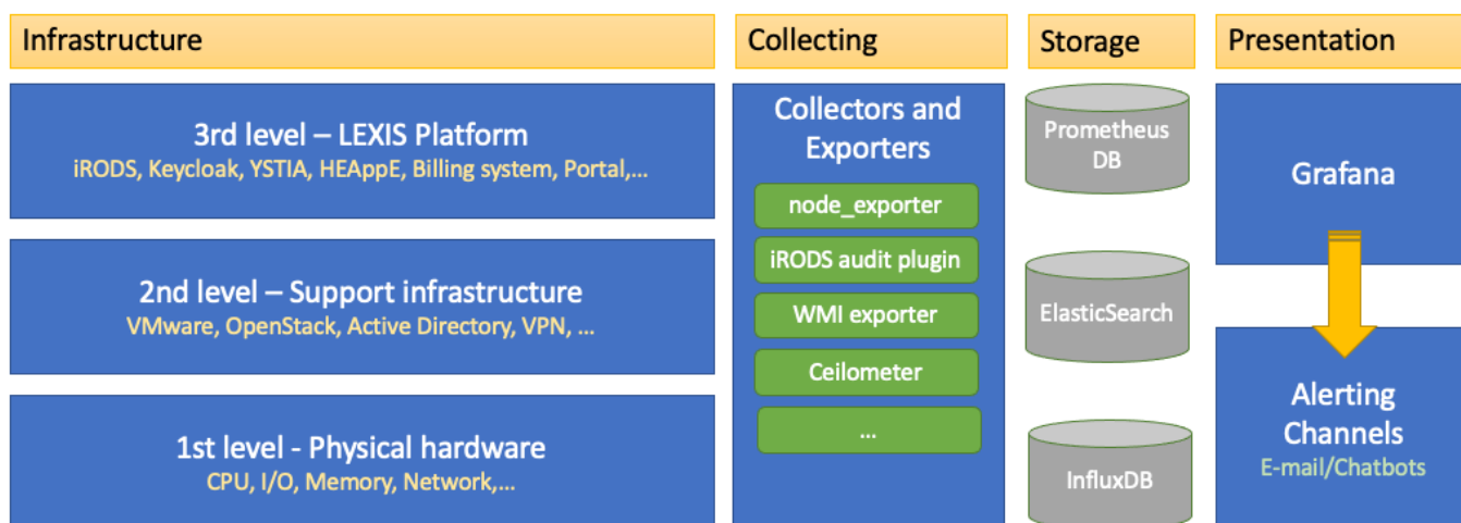
Figure 1: Levels of the LEXIS Monitoring System
