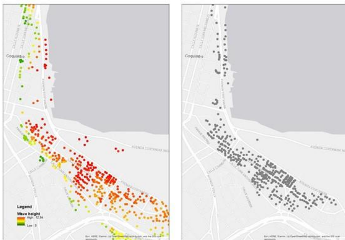
Figure 10 Buildings potentially affected by inundation on the left and results from damage surveys completed in the field after the event. Buildings affected can be detected for higher wave height simulation.
