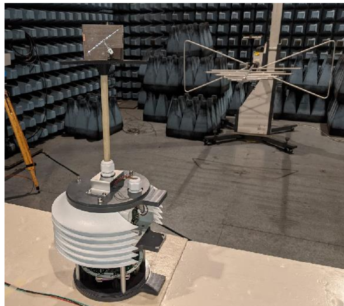
Figure 62 - Characterization in the anechoic chamber of the weather station with E-Field sensor
