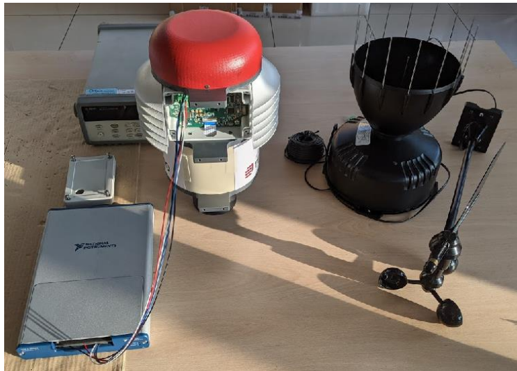
Figure 65 - The weather station and the USB-6366 Multifunction DAQ
