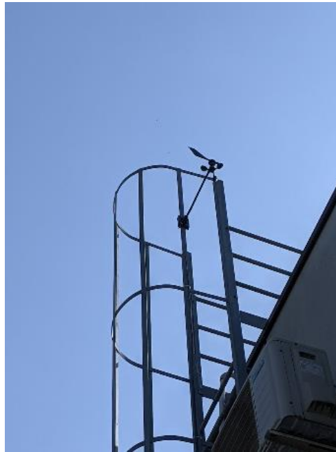
Figure 70 - Wind sensor installation
