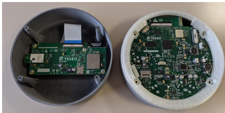
Figure 16 - Desktop assembly of the Smart Gateway
