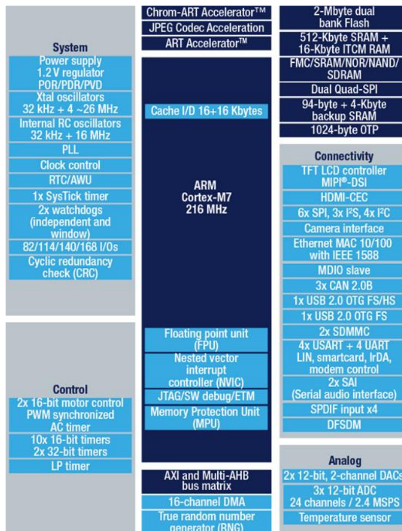
Figure 20 - STM32H769 Cortex M7 MCU Block Diagram
