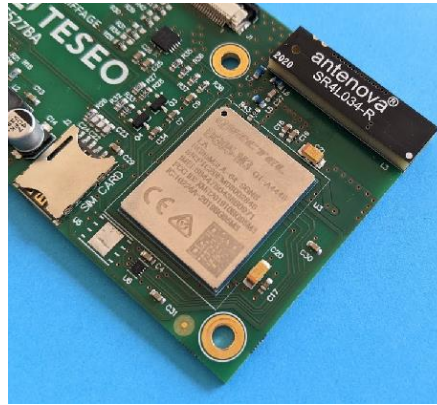
Figure 42 - GSM module and antenna implementation on the Wireless Daughterboard
