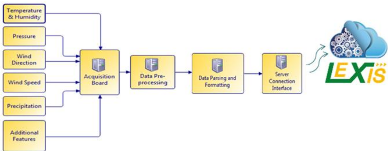
Figure 55 - Main application data flow
