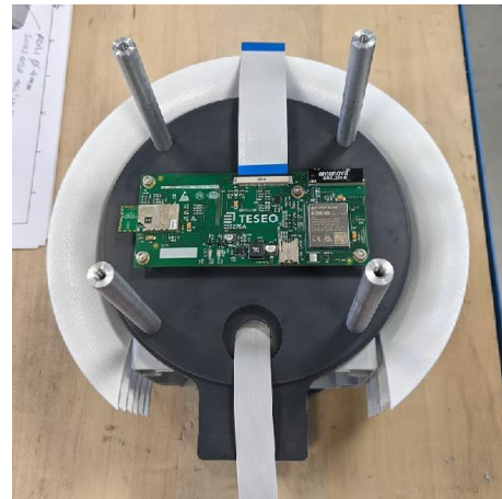
Figure 12 - Installing the wireless board
