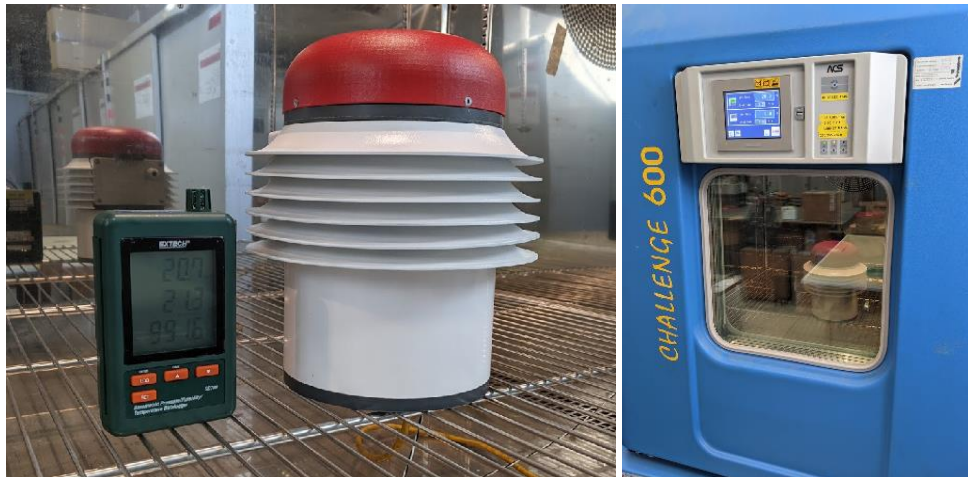
Figure 67 - The weather station into the climatic chamber at TESEO premises
