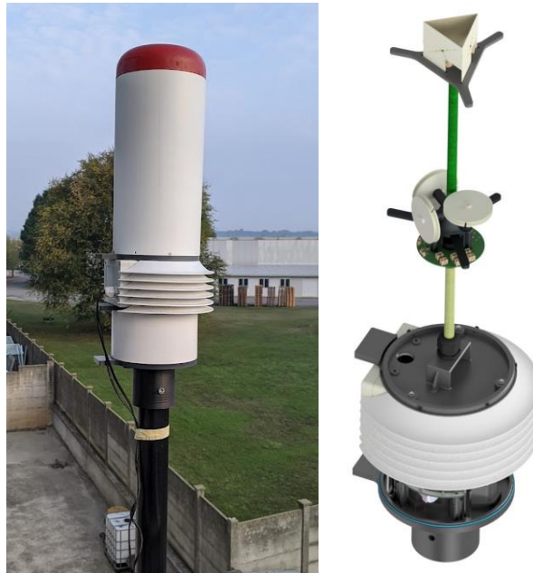
Figure 2 Smart Gateway integrated in the weather station with Electric Field monitor (see for details Deliverable D7.7 [4])
